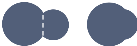
Figure 2.10-2: Left object is divided into two objects by the white boundary while the right object remains a single object when the Split touching objects processing is applied
