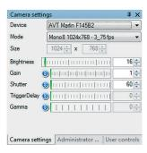
Once the IEEE1394 driver is installed, a live image can be displayed in the Aphelion™ Lab interface within a few seconds. The user has only to select the right camera configuration settings and adjust the exposure parameters to acquire high-quality images.
