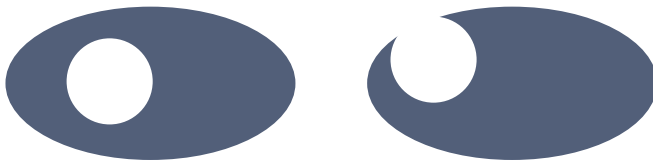
Figure 2.9-1: Left object includes one hole. Right object has no hole because the white area inside the object is not totally surrounded by the object
